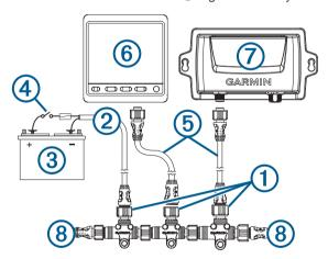
2 Connect the included NMEA 2000 power cable ② to a 9 to 12 Vdc power source ③ through a switch ④.
