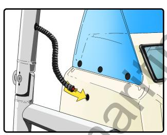
PRO TIP: We recommend covering the exposed wire with wire loom for a professional appearance.
