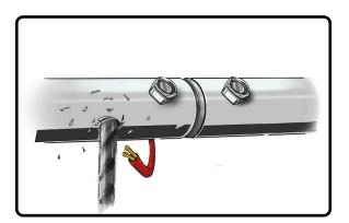
Run the wire through the frame and drilled holes
